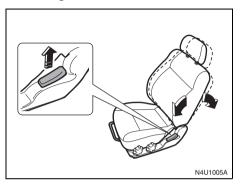
To adjust the seatback angle, lift the lever located on the outboard side of the seat and move the seatback to the desired position.
